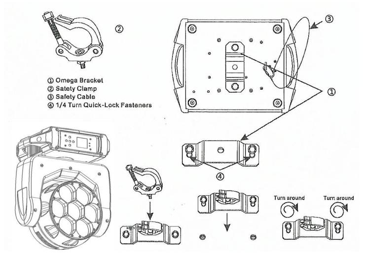
Regardless of the rigging option you choose for your Zoom wash, always be sure to secure your fixture with a safety cable. The fixture provides a built-in rigging point for a safety cable on the hanging bracket as illustrated above. Be sure to only use the designated rigging point for the safety cable and never secure a safety cable to a carrying handle.
